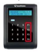
Before employees present their access cards to GV-AS1010, they can press the function keys to indicate it is the start or end of Work Time, Away, Overtime, Break Time or enter a Job Code. The attendance data are accessible in GV-TAWeb, the time and attendance system in GV-ASManager.
