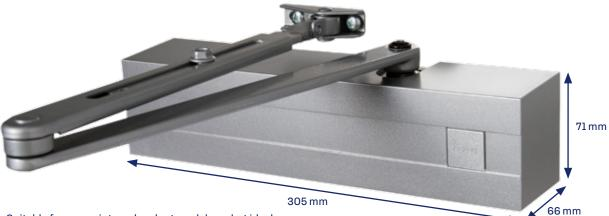
Suitable for use on internal and external doors but ideal solution for extremely heavy doors. The maximum door weight 160 kg and door leaf width 1600 mm with a standard arm installation.
