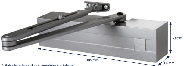
Suitable for external doors, large doors and internal doors exposed to conditions of pressure and heavy use. The maximum door weight 120 kg, and door leaf width 1400 mm with a standard arm installation. When installed with a guide rail maximum door weight is 80 kg and door leaf width is 1100 mm.
