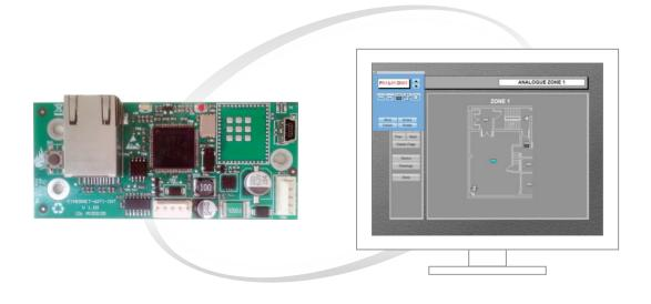
GFE-TCP-ODY is a new interface for TCP/IP communication, for integration of JUNIOR V4 and ORION-PLUS panels into ODYSSEY XL software. It uses our advanced communication protocol to send and receive information from panel, enabling complete supervision over the most complex fire detection systems.
