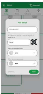
Before scanning the QR code on the sensor Press the Add Device button. Type the requested data.
