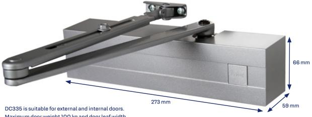
Maximum door weight 100 kg and door leaf width 1250 mm with a standard arm installation.
