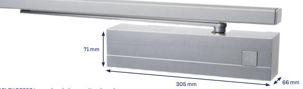
ABLOY DC250 is non-handed cam action door closer and therefore very easy to install. Thanks to the cam construction it is extremely light to open, yet in terms of closing force strong enough for heavy duty applications. Suitable for external and internal doors. Compatible with ABLOY FD460 series fire door closing systems. Maximum door weight 120 kg and door leaf width 1400 mm with guide rail installation.
