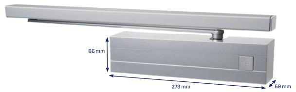
Non-handed cam action door closer. Thanks to CAM it is light to open but still strong enough to close the door in every situation. DC330 can be adjusted to meet the requirements of the light opening resistance, for example the EA (Equality Act) in UK. Suitable for external and internal doors. The maximum door weight 80 kg and door leaf width 1100 mm with a guide rail installation.
